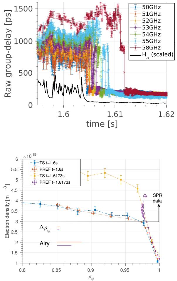
Figure 2: SPR density profile in O-mode during L-H mode transition shot 61337. (a) Raw group-delay with  $8.75\mu\text{s}$  averaging. (b) Comparison with TS with  $8.75\mu\text{s}$  averaging.
