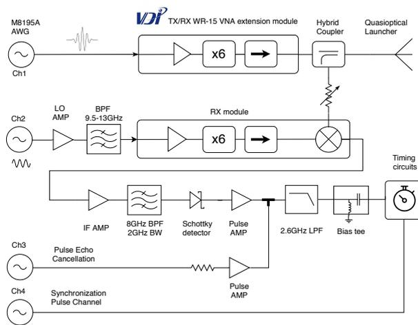
Figure 1: SPR schematic diagram
