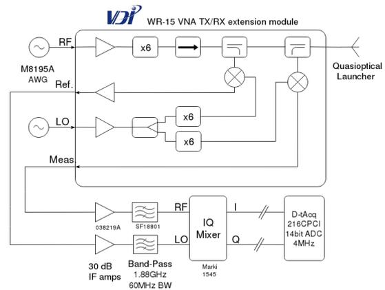
Figure 1: Block diagram of the sweepable single-frequency DBS implementation
