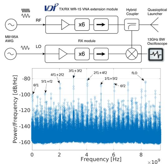
Figure 2: Top: Block diagram of the multi-channel DBS setup. Bottom: raw IF PSD spectra showing the main multiplication and intermodulation terms.
