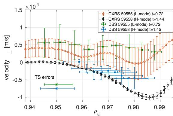
Figure 3: Comparing DBS perpendicular turbulence velocity estimates with CXRS  $v_{\text{ExB}}$  estimates in L-mode (59555,  $k_{\perp}$  5-5.8  $\text{cm}^{-1}$ ) and H-mode (59558,  $k_{\perp}$  6.5-7.5  $\text{cm}^{-1}$ ) discharges. The average TS contribution to  $\Delta\rho_{\psi}$  and  $\Delta v$  are shown decoupled from the inherent DBS uncertainties for illustrative purposes.
